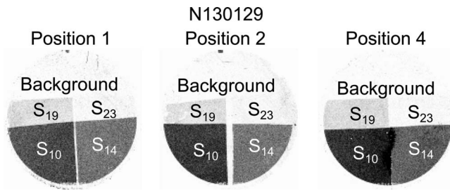
FIG. 8. DD-proton signal obtained at three different detector positions using the “thick” SRF (10, 14, 19, 23- \mu\text{m} Ta filters) on NIF direct-drive \text{D}_2 -filled thin-glass shell shot N130129. Dark signifies a greater proton fluence. A similar absolute fluence level and ratio of proton signals is observed at each detector. The gradation in fluence across the different windows, with a finite fraction of the proton spectrum permitted behind multiple windows, indicates a fairly broad proton spectrum.
